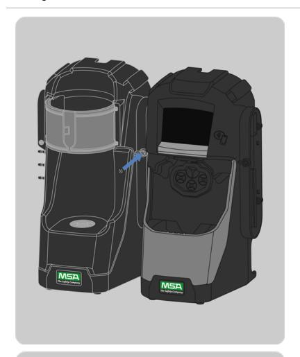
3. With the first Cylinder Holder on the left and the first Test Stand on the right, align the barbed connectors and fittings, and firmly push the two units together until the screw holes in the flange align.
