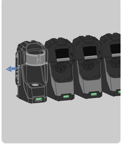
11. Remove the top barbed connector from the left most cylinder holder.
