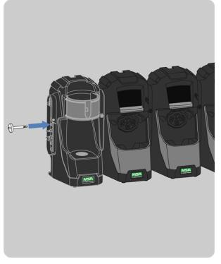
3. Insert the new filter and tube onto the same barb fitting of the fresh air port.
