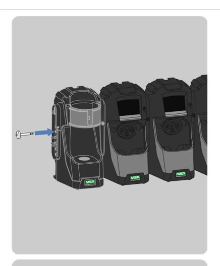
12. Install the Fresh Air Filter into the top port of the left most Cylinder Holder.
