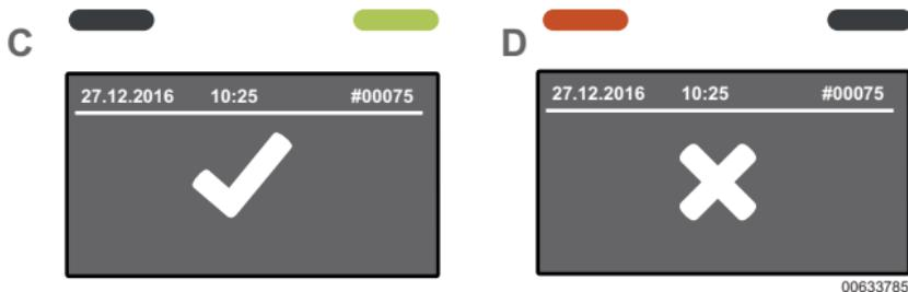
**C)** No alcohol detected. The test is passed. Additionally, the green LED is lit. After 2 sec. the instrument will be ready for use again.
