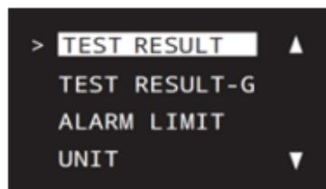
The test results can be checked under the "TEST RESULT" tab. The test number, test result, date and time are also saved. The last test result is displayed first.
